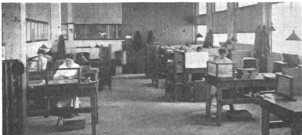
SCIENTIFIC STUDY OF MATERIALS AND WASTE DICTATED THE ARRANGEMENT OF THIS BINDERY THE GLASS SCREENS PROTECTING THE DESKS AT WHICH GOLD LEAF IS APPLIED EFFECT A LARGE SAVING OF GOLD EACH YEAR
