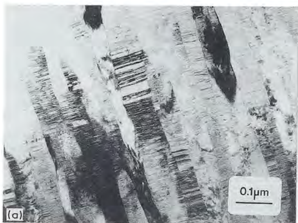
Figure 2 (a) Transmission electron micrograph showing the morphology of columns, twins, and stacking faults in as-sputtered Inconel 617. (b) Higher magnification transmission micrograph illustrating the high density and fineness of planar defects.
