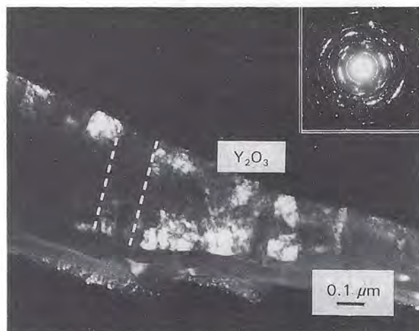
Figure 8 Transmission electron micrograph of a portion of the Y_2O_3 coating and selected-area electron diffraction pattern (inset) from a TiAl/Nb laminate. Note the grains remain columnar after hot-pressing at 1066 °C for 4 h.
