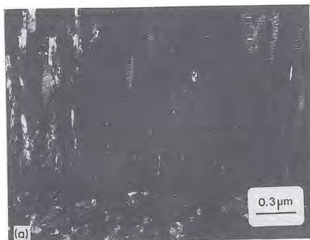
Figure 4 (a) Dark-field transmission electron micrograph of the diffusion spot labelled "A" in Fig. 3. (b) Dark field transmission electron micrograph of the diffraction spot labelled "B" in Fig. 3, showing that streaking is due to \{111\} planar defects.
