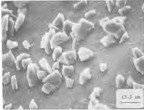
Fig. 2. Scanning electron micrograph of SiC erodent: note the range of particle sizes and shapes; 45° tilt.
