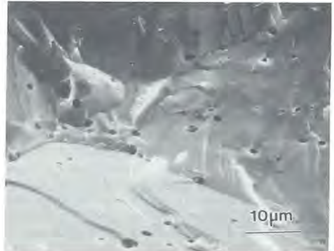
Fig. 4. Fractograph of \text{CrB}_2 showing failure by cleavage. Unconnected porosity and \text{AlSi}_x\text{O}_y inclusions are apparent. The grain size is 20\text{--}30 \mu\text{m} . The density of hot-pressed \text{CrB}_2 is approximately 88% of theoretical.
