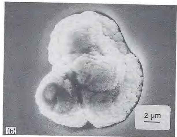
Figure 3 (a) Scanning electron micrograph of a nodular growth defect in sputtered Inconel 617 deposited on to ground \alpha -titanium. Note that the coating has fractured around the growth defect in this bend test sample. (b) Scanning electron micrograph of a nodular growth defect in sputtered Inconel 617 deposited on to polished \alpha -titanium. Note the smooth surface finish around the nodule.
