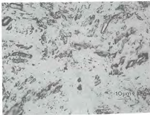
Fig. 1. Light micrograph of polished hot-pressed \text{CrB}_2 . Pull-out appears as acicular regions. Porosity is not evident in this micrograph.
