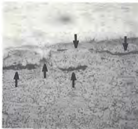
Figure 8: This photo, from the fork blade-dropout joint of another custom American frame, shows that filler metal inclusion doesn't affect just brass-brazed frames. The arrows point to areas where BA9-1 has entered the grains of Reynolds 531. The maximum depth of the inclusions is only about 4.5% of the thickness of the tube. Overheating the brazing alloy will result in much deeper filler metal inclusions (magnified 240 times).
