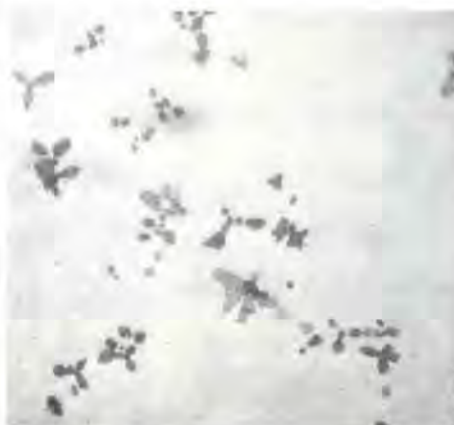
Figure 6: These flower-like crystals were found in the fork crown joint of a well-known production Italian racing frame. The filler metal is an (R)BCuZn-type, and the base metal is Columbus SL. The average diameter of the crystals is about 0.00085 inches (magnified 240 times).
