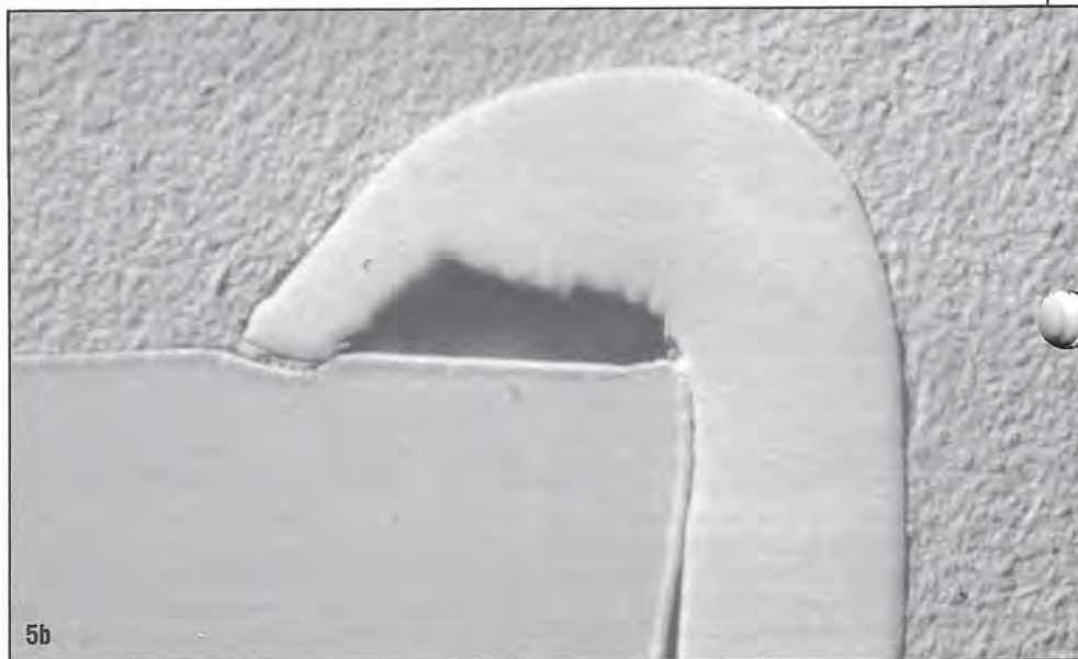
Figure 5: A cross section of the Synthesis rim at the spoke hole showed the oxide layer was cracked where the ferrule contacted the rim (Figure 5a, 500 times magnification). The cracked oxide layer is arrowed in Figure 5b (50 times magnification). Figure 5c is a schematic diagram showing the cross section investigated.
