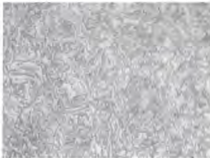
Figure 5: Reynolds 531 brazed at 1700°F for five minutes and air-cooled. This microstructure represents a slightly stronger steel than that shown in either Figure 1 or 2, since air cooling is fast enough to trap some carbon atoms in the room temperature arrangement of iron atoms. Magnified 400 times.
