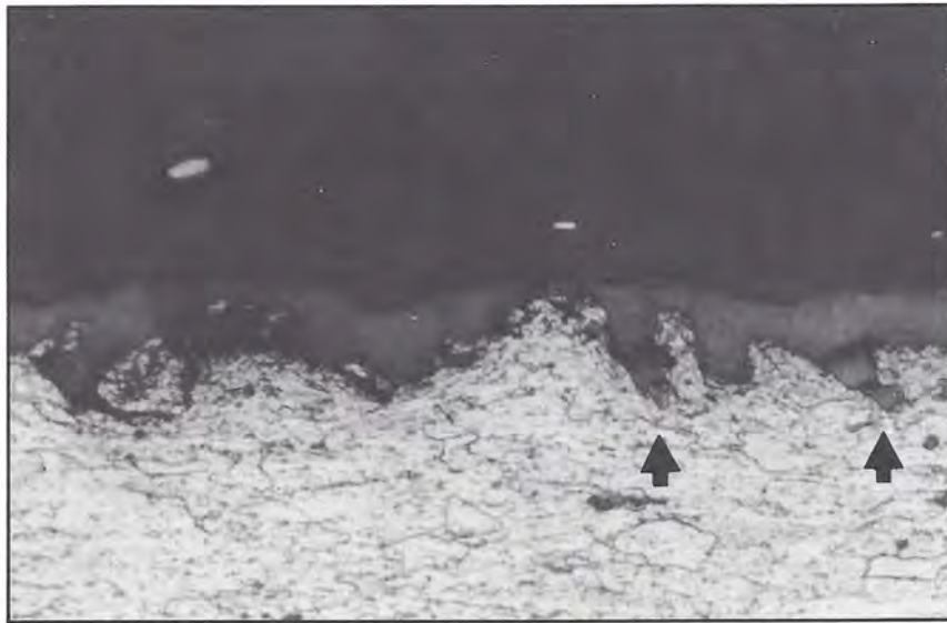
Figure 4: Deep pits like these create stress raisers that can cause fatigue failure of steel tubing.
