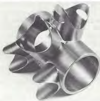
1 Track dropout of 6A1-4V titanium brazed with titanium-copper-nickel in vacuum.
