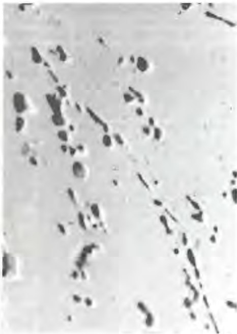
Figure 3: This photo is from the top tube/head tube joint of a well-known Italian racing frame. The porosity in the joint was caused by overheating the filler metal, an (R)BCuZn-type. If enough of these voids are present, the mechanical properties of the joint will be impaired.
