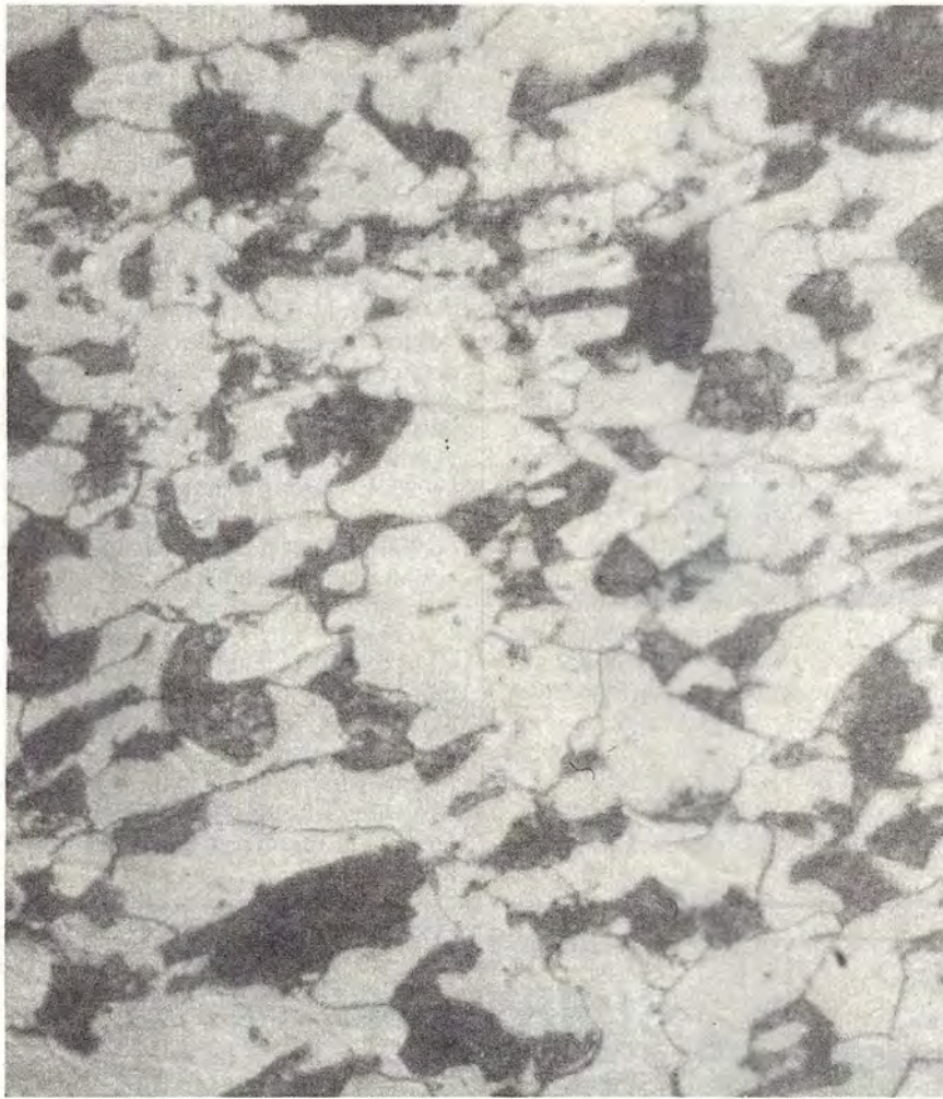
Figure 6: This is a photomicrograph of the kind of microstructure plain low-carbon steels have, and is also the type many low-alloy steels have. The dark islands are clusters of carbides, while the light areas are primarily iron. Note the individual crystals, or grains, which make up the steel's structure (800 times magnification).
