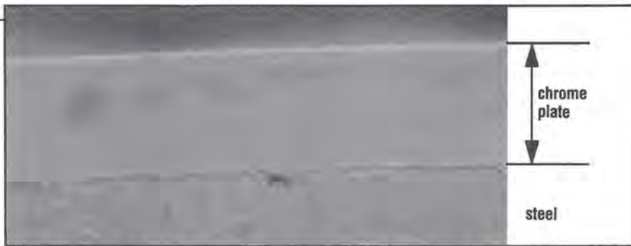
Figure 7: This is a cross section of a seat stay from a Japanese frame. The chrome is plated directly on top of the steel. The plate is about 16 microns thick, and is not cracked. 1435 times magnification.
