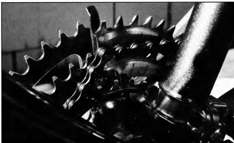
Figure 10: Bowed teeth on the swing sector for the ATB/touring model are needed to accommodate wide chain angles due to shifting on the multi-gear freewheel.
