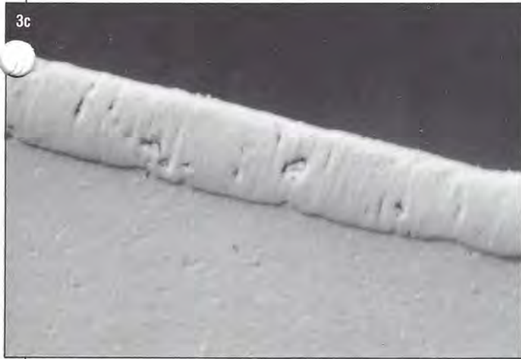
Figure 3: The hard-anodized layers of the SSC (3a), Ekip (3b), and Synthesis (3c) are 0.014-0.026-millimeter thick. The Red Label rim (3d) is not anodized. 500 times magnification.
