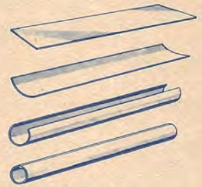
Figure 1: Seamed tubes are made by rolling a flat strip of steel into the shape of a tube and then butt welding the joint. The finished tube has a noticeable seam, characteristic of inexpensive tubing.
