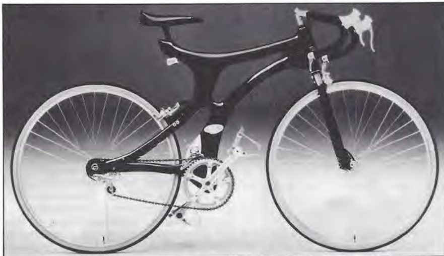
Dan Darancou's prototype: a Kevlar mat lay-up construction with a flat carbon fiber layer in the center plane.
