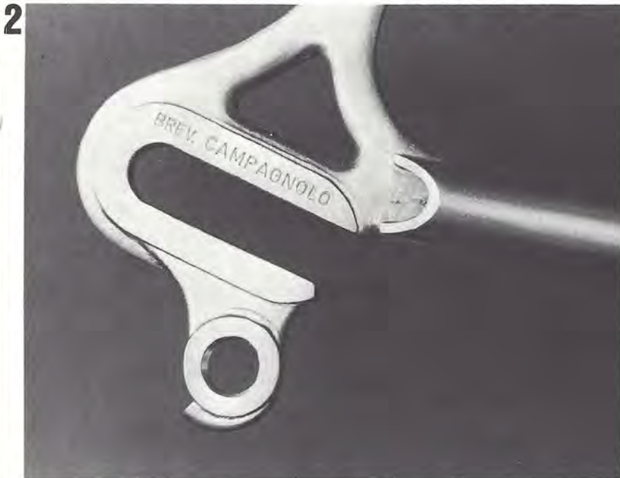
1 Track dropout of 6A1-4V titanium brazed with titanium-copper-nickel in vacuum.
